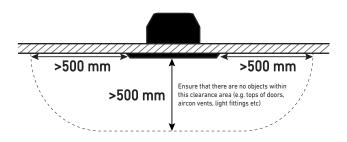
Figure 2: Soteria Dimension Optical Detector Siting Requirements (Correct Alignment)
