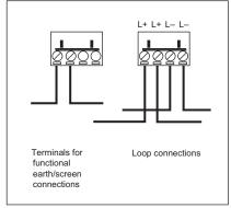
Fig 2 Terminal block connections
