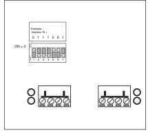
Fig 4 Terminal blocks fitted and address 78 set
